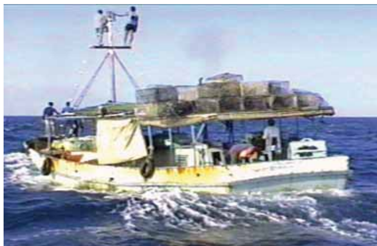
FIGURE 6 Ferrocement vessel used in the finfish fishery
